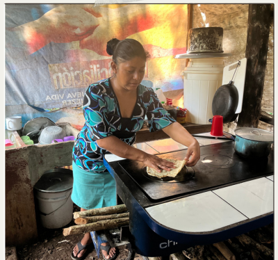
Chispa stoves burn more efficiently and safely than the typical open fire method of Guatemalan cooking
